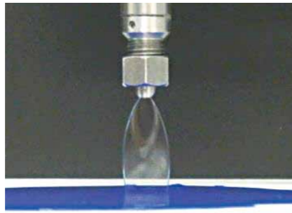
Discharge state of ELEP COAT : Curtain coating nozzle
